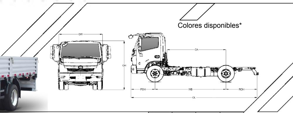
OL Largo (mm), OW Ancho total (mm), OH Altura total (mm), WB Distancia entre ejes (mm).
